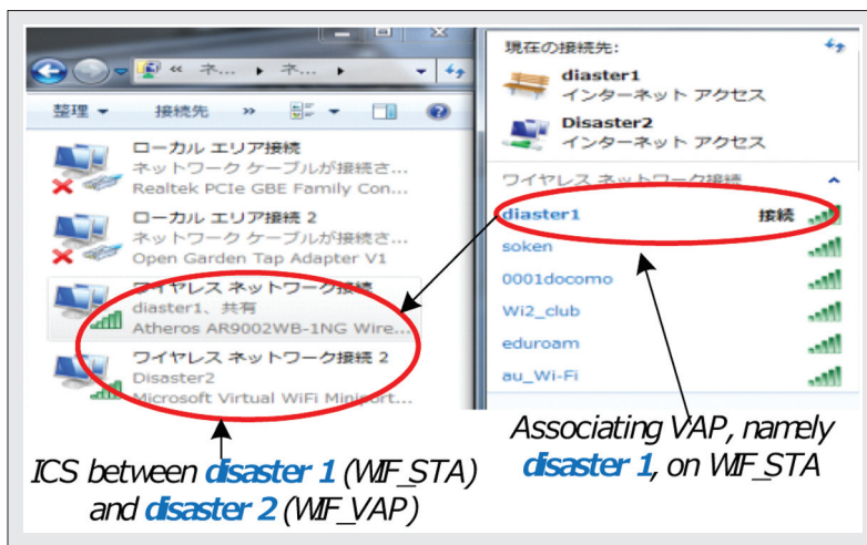
Figure 4. Internet connection sharing between the primary Internet connected WIF (disaster 1) and the secondary WIF (disaster 2).
