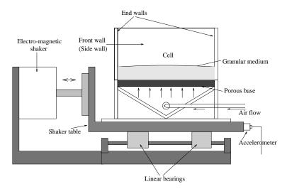
Fig. 1. – Schematic of the apparatus. The cell is made of Plexiglas, and is mounted on a Plexiglas base of the same cross-sectional dimensions which is attached to a table. An electro-mechanical actuator, driven by a sinusoidal AC signal, provides the horizontal driving.
