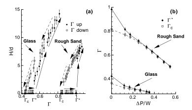
Fig. 3. – (a) Thickness of the liquefied layer next to the side walls  $(x-y \text{ plane}) vs. \Gamma$  for glass beads, d=0.6 mm and rough sand  $d_{\text{ave}}=0.6 \text{ mm}$ .  $\Gamma^*$  and  $\Gamma_c$  are the bifurcation points when  $\Gamma$  is increased and decreased quasi-statically. (b) Bifurcation points  $\Gamma^*$  and  $\Gamma_c vs.$  dimensionless lifting pressure.
