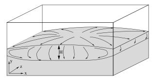
Fig. 2. – Sketch of time-averaged convection flow lines in the liquified layer. Magnitude of the flow in y and z directions has been greatly exaggerated.
