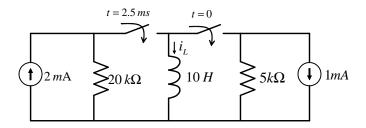
Consider the circuit in the figure in which the initial energy stored in the inductor is zero. 1.a) Find  $i_L(t)$  for  $0 \le t \le 2.5 ms$ .
