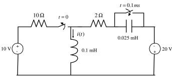
**3.** (4 points) Consider the circuit in the figure, where the first switch opens at time t = 0 after a long time, and the second switch closes at time t = 0.1 ms. We refer to the current in the inductor as i(t) (see figure).
