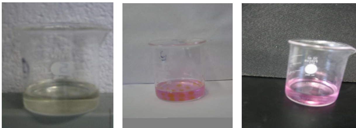
Figure 9 (a) Unreacted soap solution, (b) Hazy pink solution with unreacted oil, (c) Clear pink solution indicating the formation of soap.
