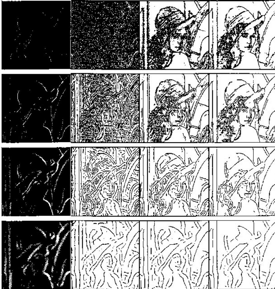
Fig. 8: The first column gives the modulus images M_{2^j}f(x,y) for 1 \leq j \leq 4 of the lady image shown at the top left of fig. 9. The second column displays the position of the maxima of M_{2^j}f(x,y) . The third and fourth columns display the position of the local maxima whose amplitude are respectively larger than 4 and 8. The maxima that have been removed correspond essentially to the noise and the light texture irregularities.
