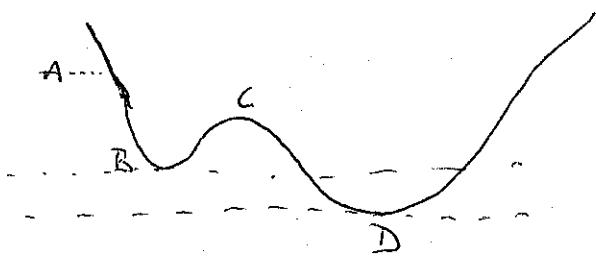
Depending on the starting location and velocity, the ball will exhibit various dynamics. But energy will be conserved since there is no friction. Thus a ball released at A with 0 velocity will roll down the hill, pass B, up to C, over that hill, pass D and make it to the same height as A, but now on the right side of the landscape. It will then turn around and repeat. If  $\mathbf{P}$  measures location and  $\mathbf{g} = \mathbf{p}'$  measures velocity, the phase portrait is
