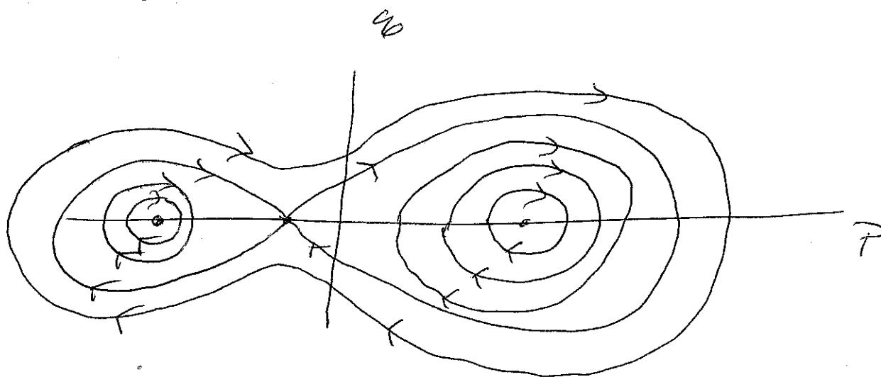
This phase portrait has 2 centers corresponding to the local minima at B and D, a saddle point corresponding to the local maxima at C. There are periodic orbits surrounding the centers and homoclinic orbits connecting the saddle to itself. The origin of the  $(P_1 z)$  plane is arbitrarily chosen. Thus given an energy landscape, we can easily find the phase portrait and vice versa.
