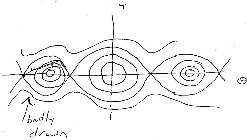
This graph shows that solutions either lie at critical or distinct fixed points, along closed orbits, or along curves that connect distinct fixed points. We need to add the direction or vector field to complete the picture.
