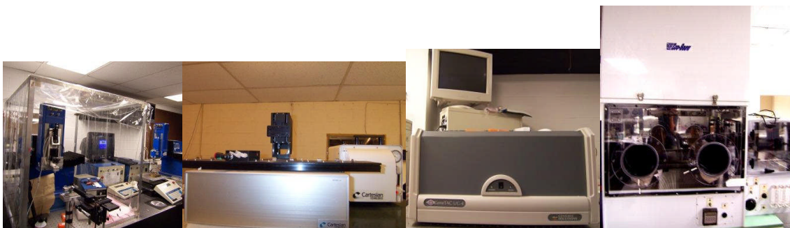
Figure 3c: Realtime Lab Microarray facilities, left to light: Smartpin on XY-300 robot, Cartesian Microarrayer, GeneTAC UC4 scanner, EcoSnow process station.
