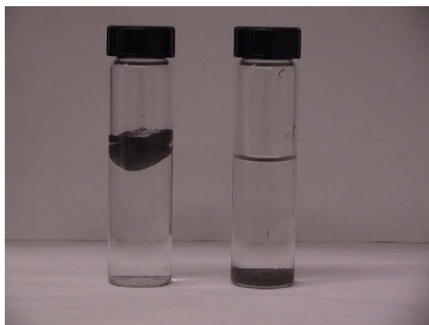
Fig. 6. Ground magnesium powder settled in water (right) while the coated sample floated on water (left) even after 30 days of exposure to the atmosphere.
