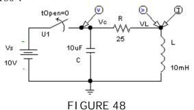
To set the switches attributes, double click on the switch part to open its Attribute window, shown in Figure 49. Parameters of interest are
