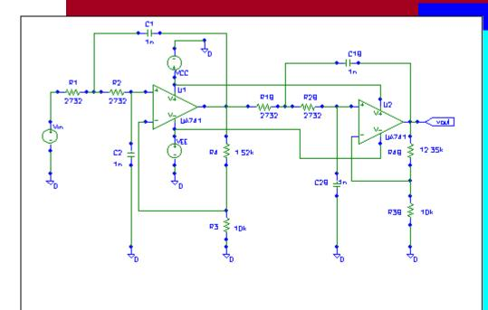
\* Schematics Netlist X U1 \$N 0002 \$N 0003 \$N\_0004 \$N\_0005 \$N\_0001 **UA741** V\_VCC \$N\_0004 0 dc 10 V VEE \$N 0005 0 dc -10 V\_Vin \$N\_0006 0 dc 0 ac 1 R\_R1 \$N\_0006 \$N\_0007 2732 \$N 0007 \$N 0002 2732 R R2 R R4 \$N 0003 \$N 0001 1.52k R R3 0 \$N 0003 10k  $C_C1$ \$N\_0007 \$N\_0001 1n  $C_C2$ 0 \$N\_0002 1n \$N\_0008 \$N\_0009 X\_U2 \$N\_0004 \$N\_0005 vout UA741 R\_R1B \$N\_0001 \$N\_0010 2732 R R2B \$N 0010 \$N 0008 2732
