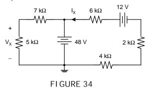
Your simulation should yield,  $V_X = 20 \text{ V}$  and  $I_X = -3.0 \text{ mA}$ . Of course, the negative sign on the current means the direction of flow is opposite its defined direction in Figure 34.
