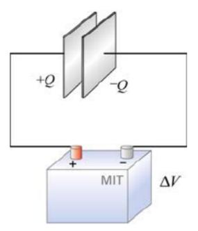
The connection results in sharing the charges between the terminals and the plates
