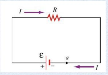
Simple circuit: battery + resistor
