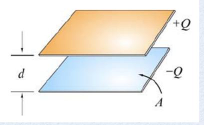
The amount of charge Q stored in a capacitor is proportional to ΔV (the electric potential difference between the plates)
