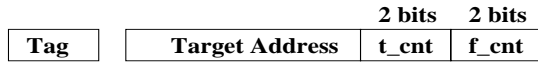
Figure 2. The structure of extended BTB entry (A tagged BTB is used in this paper).
