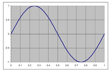
In the following figure, the same sine wave is displayed; however, the **Volts/Div** is set to 1 volt/division.
