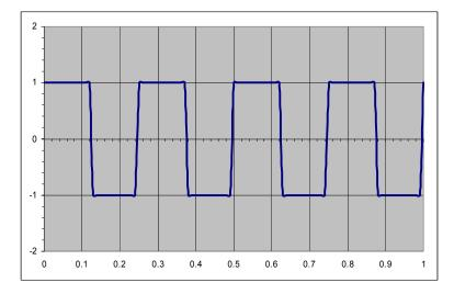
The following figure shows the trace of a square wave with a frequency of 4 Hz.
