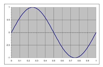
Setting the **Timebase** to 200 milliseconds/division X 10 divisions = 2 seconds will yield a display of 2 cycles.
