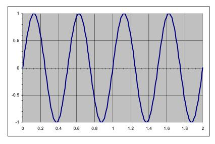
As stated previously, increasing the **Timebase** further will display more cycles. However, to display one cycle of the 2 Hz sine wave, the **Timebase** needs to be reduced to 50 milliseconds/division (since the inverse of the frequency 2 Hz = 0.5 seconds is the signal's period and since our scope has 10 divisions, we have 50 milliseconds).
