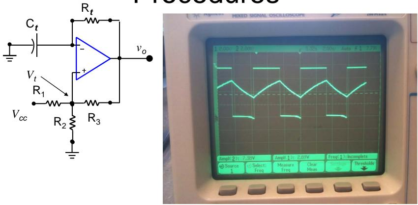
3. If the ST works, now connect the RC network and view the voltage across the output and the capacitor. They should be identical or close to the photo attached. The values of output voltages should correspond to the output voltages in 2.b) and 2.d) and the capacitor max and min voltages should correspond to the threshold values also found in 2.b) and 2.d)
