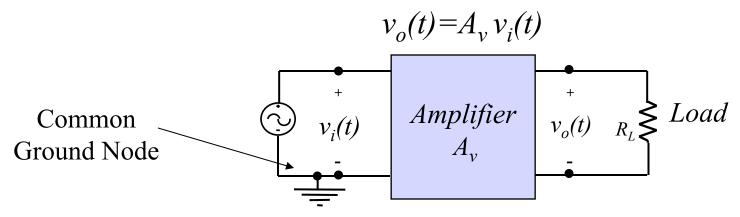
•  $A_v$  is called the voltage gain and if <0 then the amplifier is inverting; otherwise non-inverting.
