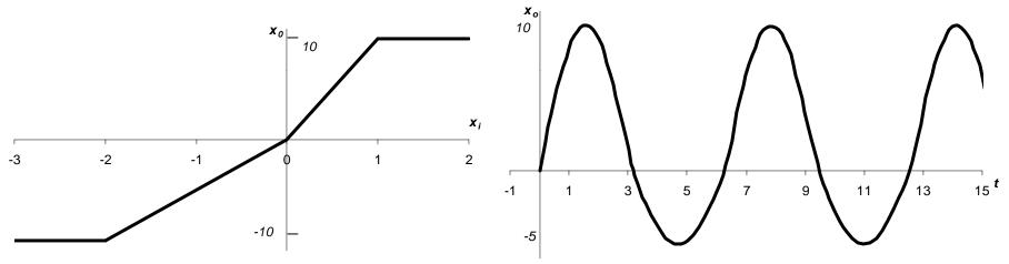
• If we want to reduce this distortion with an amplifier of  $A_f \cong 10$  and  $\beta = .1$ , we would need to have  $A\beta >> 1$ , but A = 10 and 5.
