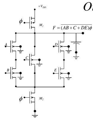
One More Example • Using this design, we can design other logic functions.
