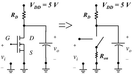
Let's find  $R_{on}$  and the pull up resistor to make the static power in the low output state to 0.25 mW. Assume  $V_{to}=1$  V,  $KP=50\mu A/V^2$ ,  $V_{OL}=.5$  V,  $V_{OH}=V_{DD}=5$  V
