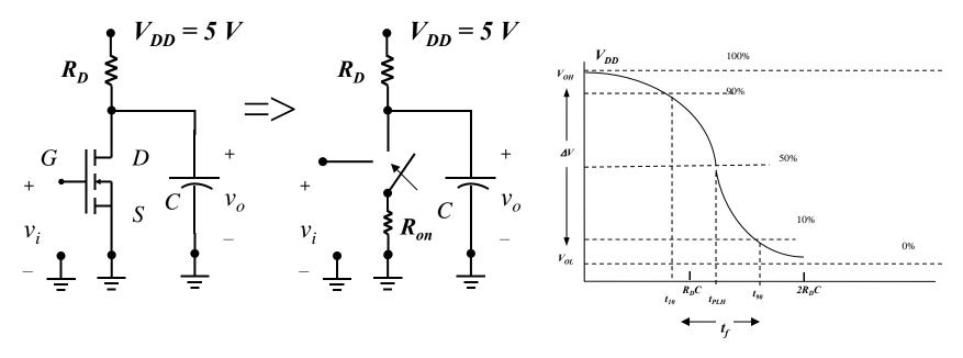
In this case, the capacitor discharges through the parallel combination of  $R_D$  and  $R_{on}$ . However, since  $R_{on} < R_D$ , the fall time from High to Low is usually shorter than the rise time from Low to High. In our example,  $R_D = 90k$  and  $R_{on} = 10k$  and the time constant for Low to High = 10kC while the time constant for High to Low is 9KC which yields 10% faster fall time than rise time. However, the overall performance is governed by the slowest time.
