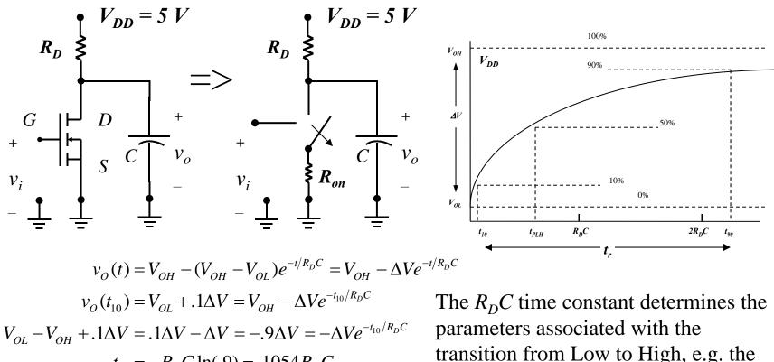
$$t_{10} = -R_D C \ln(.9) = .1054 R_D C$$
