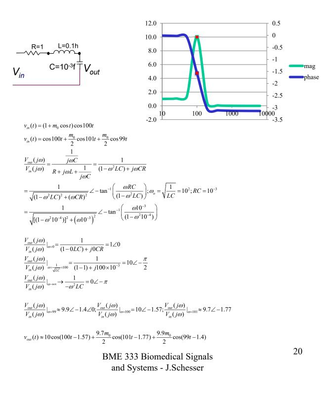
5. Calculate the Transfer Function  $V_{out}(j\omega)/V_{in}(j\omega)$  for these circuits and sketch the Bode plots:
