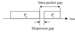
**Fig. 3** A compound probe with a heading packet ( $P_h$ ) and a trailing packet ( $P_t$ )
