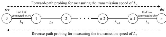
**Fig. 1** An multiple-hop end-to-end path between *src* and *dst* consisting of *n* links
