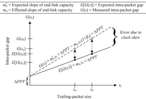
**Fig. 2** Effect of positive clock skew at node *n* in the estimation of the end-link capacity  $L_n$  using compound probes consisting of two different  $P_t$  sizes
