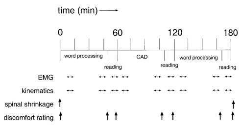
Figure 2. Schematic overview of the experimental procedures. The horizontal line represents a time axis. The experimental tasks are represented below the axis. Arrows indicate the periods during which measurements were taken.
