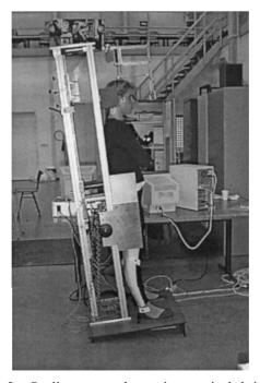
Figure 3. Stadiometer used to estimate spinal shrinkage.
