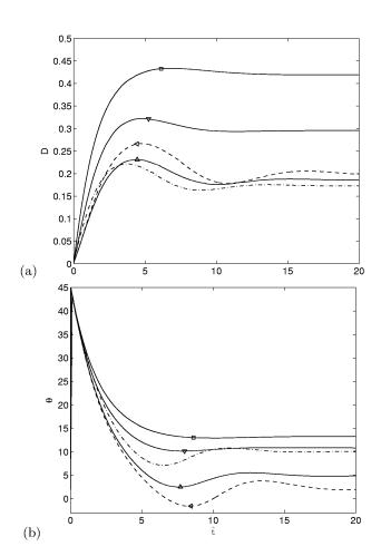
FIG. 9: (a) 3D drop deformation D and (b) drop inclination angle  $\theta$  vs. dimensionless time, for  $\lambda{=}2$  ( $\square$ ), 4 ( $\triangledown$ ), 8 ( $\triangle$ ) at fixed Ca=0.43, We=0.645, and the case  $\lambda{=}8, Ca=0.6$  ( $\triangleleft$ ). In (b), the latter case has a negative angle or an undershoot in  $\theta$  between  $\hat{t}\approx6.5$  and 10. Newtonian drop in a Newtonian matrix at Ca=0.43 and  $\lambda=8$  (-.-) is also plotted.
