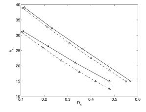
FIG. 8: Stationary state orientation angle  $\theta_s$  vs. the stationary state deformation  $D_s$ . Newtonian drop in a Newtonian matrix ( $\circ$ ) for  $\lambda=1$  and Newtonian drop in a viscoelastic matrix ( $\Delta$ ) for  $\lambda=1$  and We=0.75. 2D (-.-) and 3D (—) results are compared.
