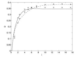
FIG. 2: Newtonian drop deformation in viscoelastic matrix. Numerical simulations at We=1 (-) and We=2 (-.-) are compared with the numerical simulations of [11], We=1 ( $\circ$ ) and We=2 ( $\triangleright$ ), at  $\lambda=1,\beta=0.5, Ca=0.3, Re=0.1$ .
