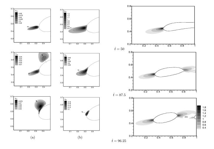
FIG. 5: Contours of extra stress tensors are compared for the (x,x), (x,z) and (z,z) components of (a) 2D, and (b) 3D simulations,  $\lambda=1,\,Ca=0.3,\,We=0.75,\,\hat{t}=4.$  Normals at the interface are indicated by straight arrows.
