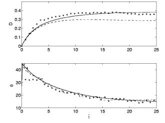
FIG. 1: Deformation (top) and angle of inclination (bottom) as a function of dimensionless time for a Newtonian drop in a viscoelastic matrix at  $\lambda=1.5,~Ca=0.36,$  and We=2.12. Experimental data from [1] (o), Oldroyd-B model simulation 3D (—) and 2D (--).
