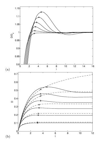
FIG. 3: Evolution of deformation for a Newtonian drop in a viscoelastic matrix at  $\lambda=1,\ We=0.75,\ Ca=0.1\ (\circ),\ 0.2\ (\Box),\ 0.3\ (\bigtriangledown),\ 0.4\ (\diamond),\ 0.5\ (\bigtriangleup),\ 0.6\ (\rhd).$  (a) 2D numerical simulations normalized by the stationary state showing relative magnitude of overshoots which increase with capillary number; (b) 2D (—) and 3D (-.-) simulations for total deformation D.
