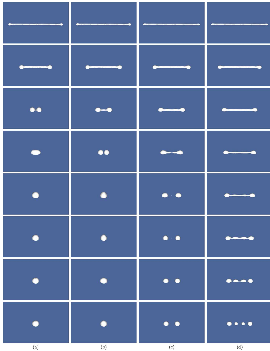
Fig. 12. Snapshots of the simulations revealing various scenarios for Oh = 0.15 and AR = 28 , and for \lambda = 1 (a), 0.1 (b), 0.01 (c), and 0 (d).
