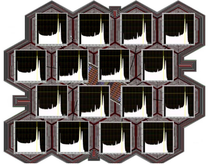
Fig. 16. Overview of ^{55}\text{Fe} spectral measurements on all 16 channels. A resolution of 152\ \text{eV} FWHM \pm 5\% was measured on the \text{Mn}_{K\alpha} line. Considering the noise from the discharge in the feedback MOSFET of the charge amplifier, this corresponds to about 84\ \text{eV} FWHM \pm 4\ \text{eV} at low energies.
