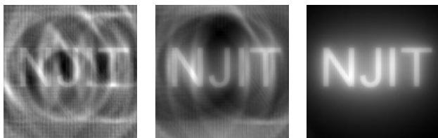
Figure 9. A THz emitting object in the shape of the NJIT logo. The number of detectors in the circular imaging array is N = 49 , N = 100 and N = 200 from left to right. The distance to the object is 25 m with a \sim 35^\circ field of view. The images are unprocessed (uncleaned). After processing to remove imaging artefacts, the image quality can be dramatically improved.
