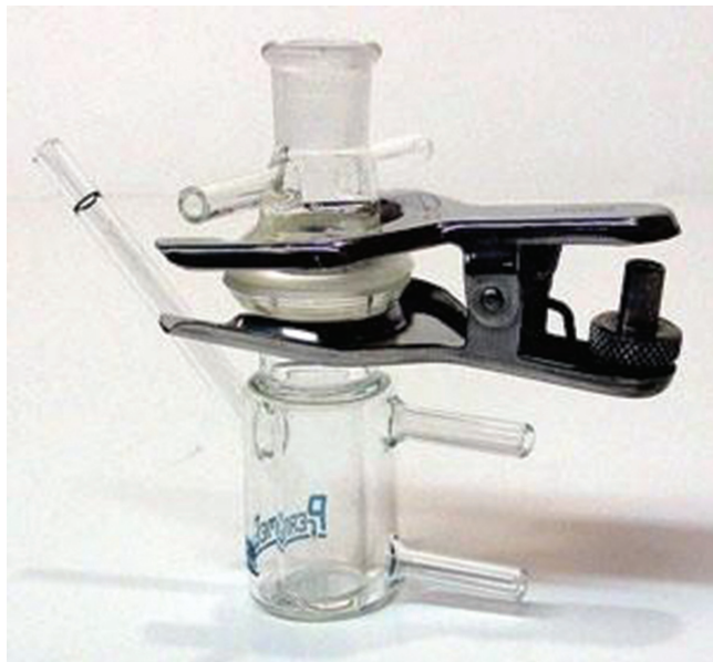
Figure 5. Fully assembled typical Franz static cell. 54
