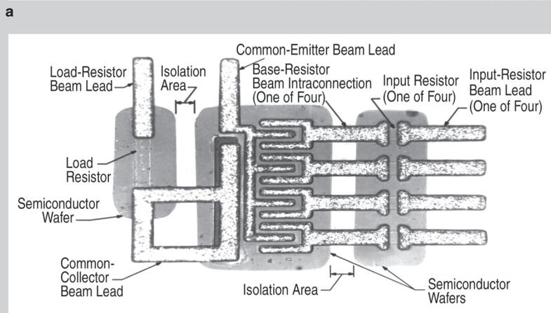
Figure 2. The top and bottom view of a four-input DCTL gate.<sup>2</sup>
