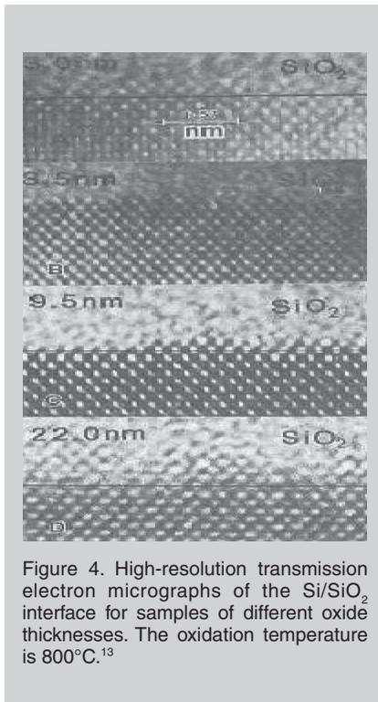
Figure 4. High-resolution transmission electron micrographs of the Si/SiO<sub>2</sub> interface for samples of different oxide thicknesses. The oxidation temperature is 800°C.<sup>13</sup>
