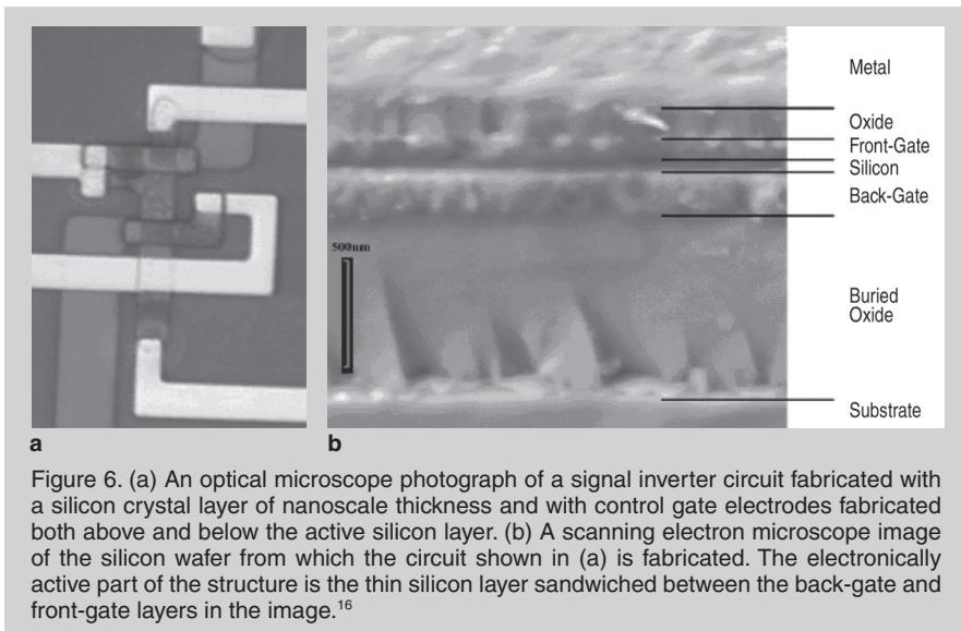
Figure 6. (a) An optical microscope photograph of a signal inverter circuit fabricated with a silicon crystal layer of nanoscale thickness and with control gate electrodes fabricated both above and below the active silicon layer. (b) A scanning electron microscope image of the silicon wafer from which the circuit shown in (a) is fabricated. The electronically active part of the structure is the thin silicon layer sandwiched between the back-gate and front-gate layers in the image.<sup>16</sup>
