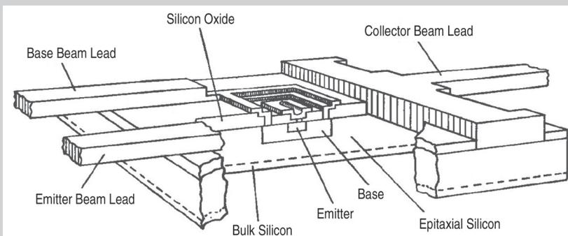
Figure 1. A cut-away cross section of high frequency beam-lead switching transistor.<sup>1</sup>
