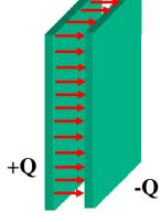
Area of each plate = ASeparation = dcharge/area =  $\sigma$ = Q/A
