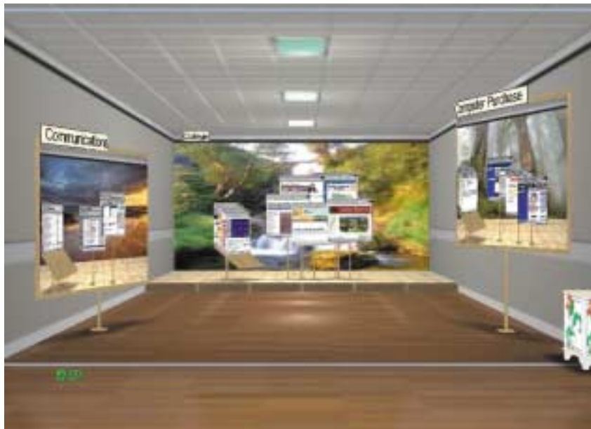
Figure 11 Microsoft's new on-screen interface called Task Gallery: 3-D graphics help users remember where they placed their documents [TRISTRAM 2001]
