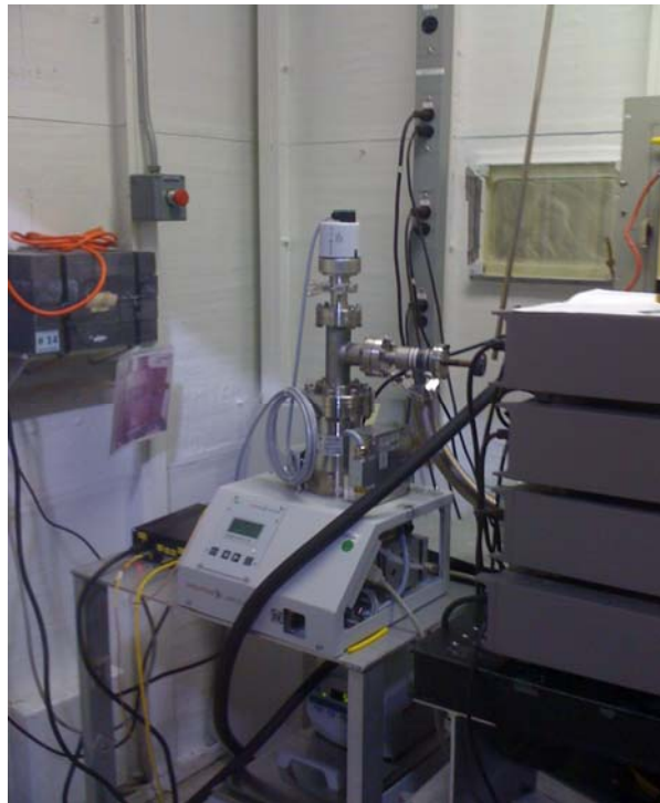
Fig. 2.4. Full set-up at X11B for detector testing first with a \text{Fe}^{55} radioactive source. Note that compact nature of the new detector in (a) and the support equipment (vacuum pump, chiller and electronic control box (black box)) in (c). The dimensions of the detector housing are 21.4 cm (length) x 14.4 cm (height) x 5.6 cm (Depth) and the weight is 8 lbs making it easily mountable for a large range of spectroscopic and scattering experiments.
