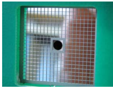
Fig.2.2. Each element (diode) is 1 mm x 1mm and the arrangement is a 20 x 20 square. There is a hole in the middle of the array for beam pass-through omitting a 4 x 4 array (hence there are 384 elements). This hole can be used for normal incidence measurements with a modified detector casing.
