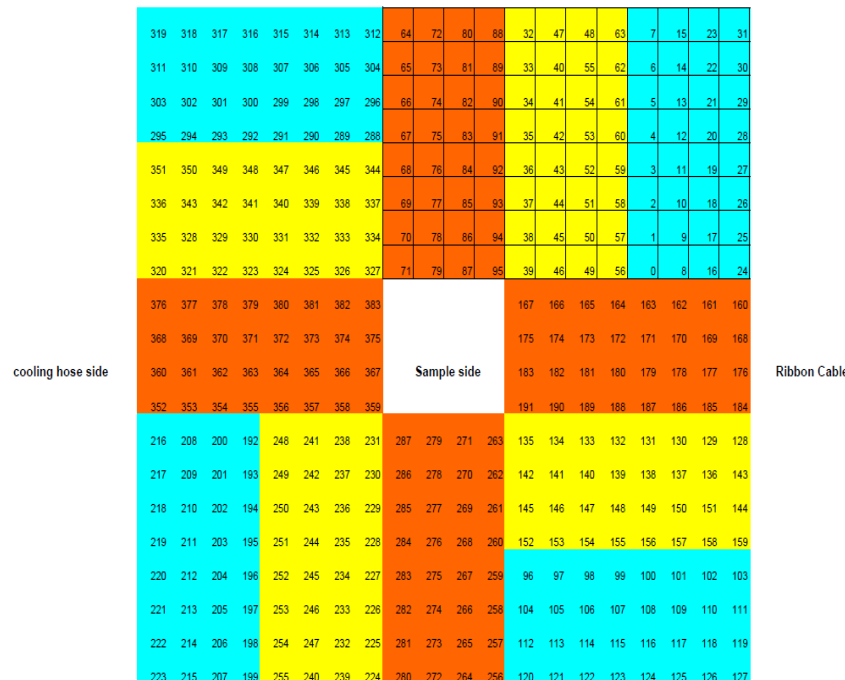
Fig. 2.3. Schematic with labels for the 384 Detector elements.
