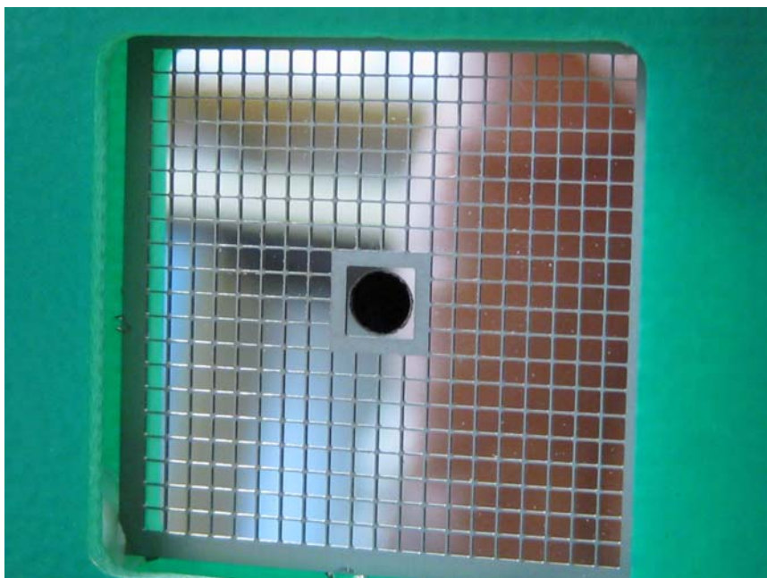
Fig. 1. View of detector showing pass through hole.
