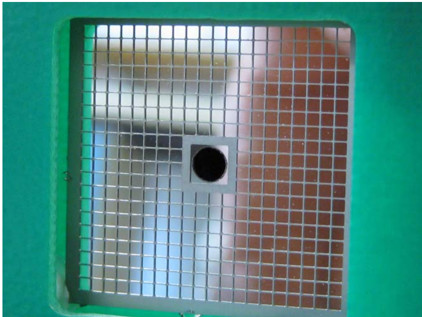
Fig. 1. View of detector showing pass through hole.
