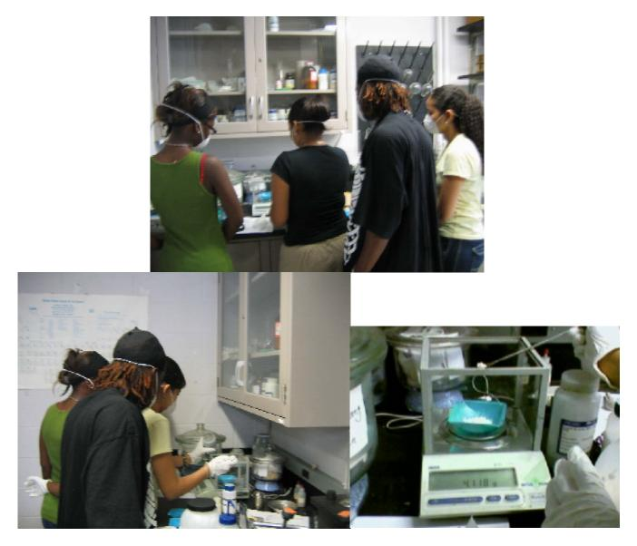
**Fig. 3**. Weighing the components ( $Y_2O_3$ , CuO and BaCO3), needed to get the correct stoichiometric ratio for YBCO ( $YBa_2Cu_3O_{6+x}$ ).
