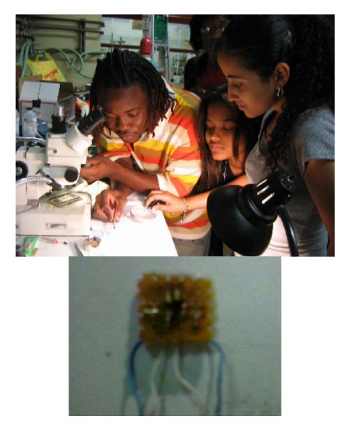
Fig. 9. Preparing a rectangular (polished) sample for Resistivity measurements. Rectangualr sample as placed on circuit board.
