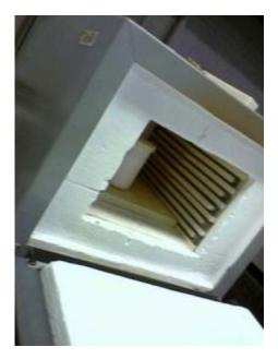
**Fig. 5**. Sample placed in Alumina crucible with lid for calcination (firing at high temperature ~ 950° C) in high temperature furnace.
