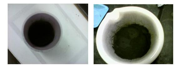
Fig. 6. Black powder obtained after several heating cycles. Sample pressed into pellet and reheated.
