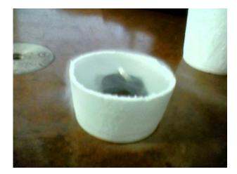
Fig. 7. Meissner effect test of pressed pellet.
