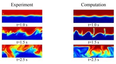
**Electrokinetic instability in microchannels.** Left: *experimental data* showing instability mixing of high (red) and low (blue) electric conductivity streams. Right: reproduction of dynamics from *numerical computations* (from Lin *et al.*, *Phys. Fluids* 16(6), 1922-1935, 2004).
