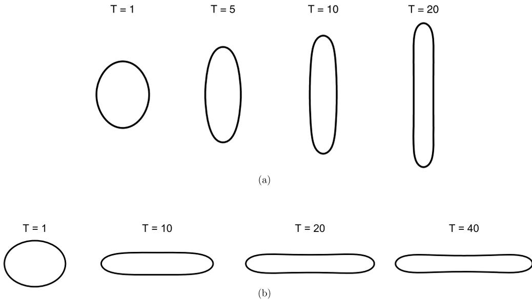
Fig. 8. Drop deformation with  $Ca_E = 2$  at different times: (a)  $\sigma_r = 10$ ,  $\epsilon_r = 1.37$ , and (b)  $\sigma_r = 0.6$ ,  $\epsilon_r = 1.37$ .
