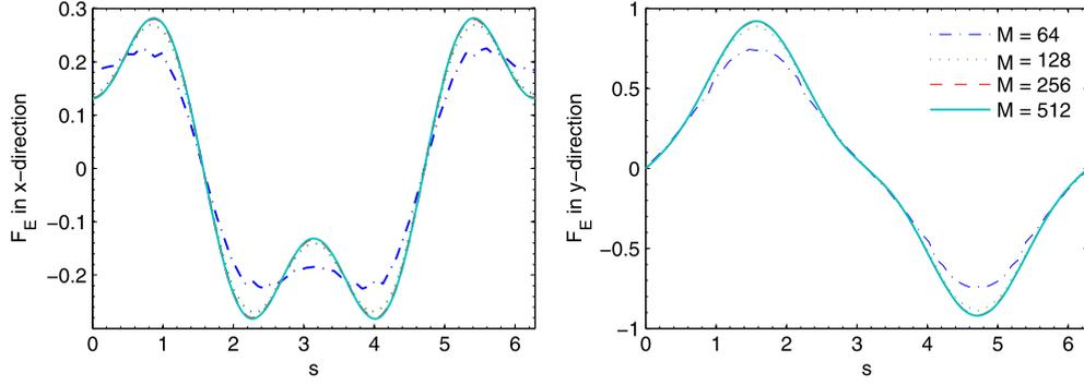
**Fig. 3.** Electric force  $\mathbf{F}_E$  at different number of markers  $M = 64, 128, 256$  and  $512$ . Left panel is the  $x$  component and right panel is the  $y$  component.  $M = 64$  for dash-dotted lines,  $M = 128$  for dotted lines,  $M = 256$  for dashed lines, and  $M = 512$  for solid lines.
