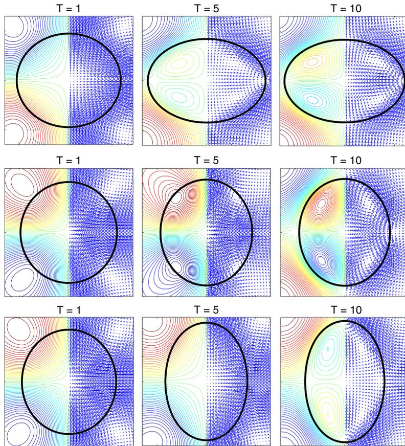
**Fig. 6.** Drop shapes and flow patterns for Cases A, B, and C at different times. Top row: Case A ( $\sigma_r = 1.75$ ,  $\varepsilon_r = 3.5$ ), oblate and clockwise; Middle row: Case B ( $\sigma_r = 3.25$ ,  $\varepsilon_r = 3.5$ ), prolate and clockwise; Bottom row: Case C ( $\sigma_r = 4.75$ ,  $\varepsilon_r = 3.5$ ), prolate and counterclockwise.  $Ca_E = 1$ .
