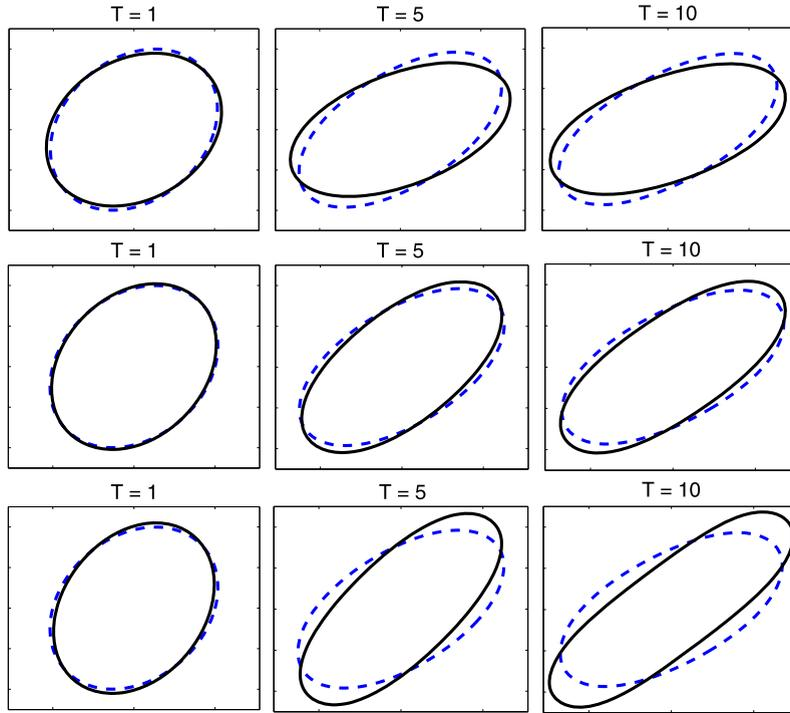
Fig. 7. The snapshots for a drop under both an electric field (vertical) and shear flow (horizontal)  $\mathbf{u} = (0.3y, 0)$  with (solid line) or without (dashed line) the electric effect. Top row: Case A; Middle row: Case B; Bottom row: Case C.  $Ca_E = 1$ .
