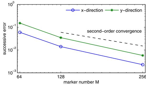
Fig. 4. The successive errors of the electric interfacial force  $F_E$  in both  $x$  and  $y$  directions (see legends). The rate of convergence is around second-order.
