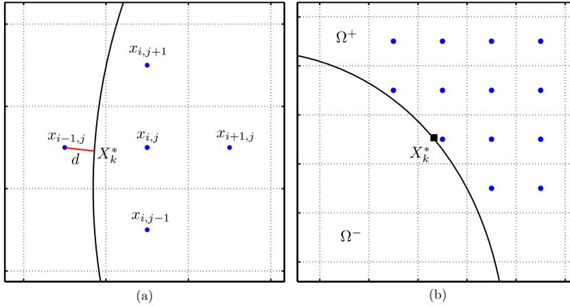
**Fig. 2.** (a) The grid points used in five-point Laplacian at the irregular point  $\mathbf{x}_{ij}$  might cross the interface. (b) A grid layout indicating the neighboring grid points used in least squares cubic polynomial approximation to the one-sided normal derivative at  $\mathbf{X}_k^*$ .
