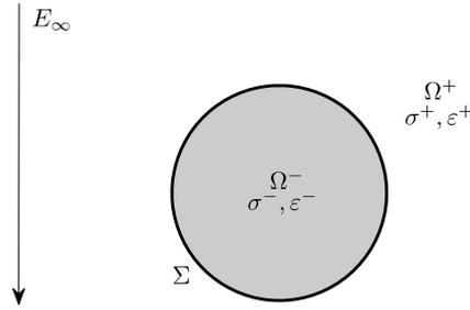
Fig. 1. A leaky dielectric drop suspended in another leaky dielectric fluid under DC electric field.
