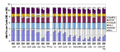
Fig. 3. Functional unit idleness/utilization comparison between DIE and SIE.
