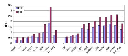
Fig. 2. Performance loss due to dual-instruction execution: DIE vs. SIE.
