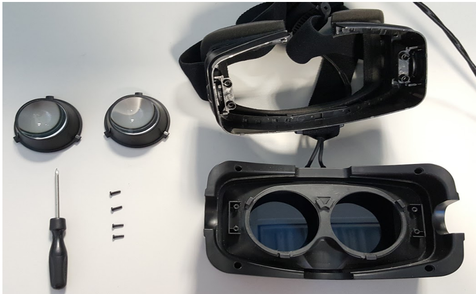
Figure 18: A fully disassembled Oculus Rift
