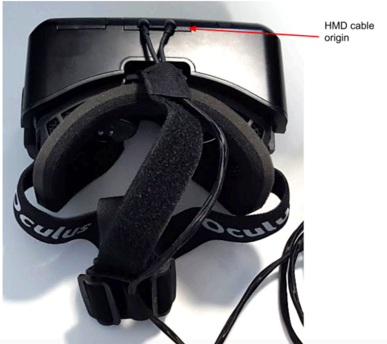
Figure 20: Top view of the HMD showing the attachment point of the fixed cable
