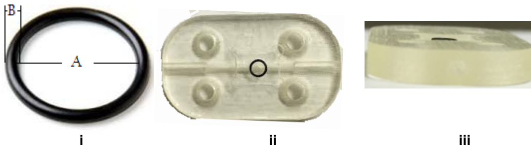
Figure 8: i) O-ring dimensions ii) o-ring in housing unit iii) 33% of o-ring exposed above groove
