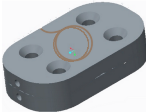
Figure 14: The inductor coil, in gold, originates from the sensor situated between the two halves of a housing unit and loops to rest on the top of the complete housing unit as shown.
