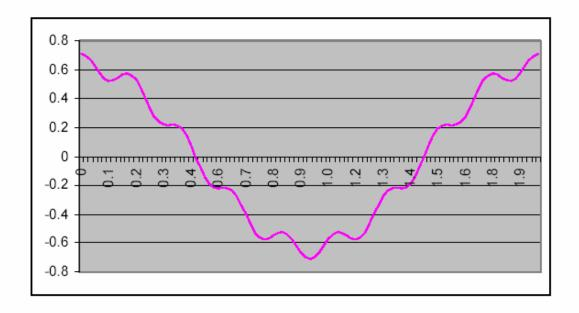
If the lowpass filter has bandwidth 3 Hz, then the first three components are passed (k=2). The resulting signal is shown below:
