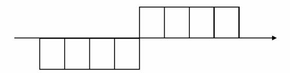
The above figure shows a sequence of 4 1s followed by 4 0s. A long sequence of 1s or a long sequence of 0s produces a long period during which there is no change in the signal level. Consequently, there are no transitions ("zero crossings") that help a synchronization circuit determine where the boundary of each signaling interval is located.
