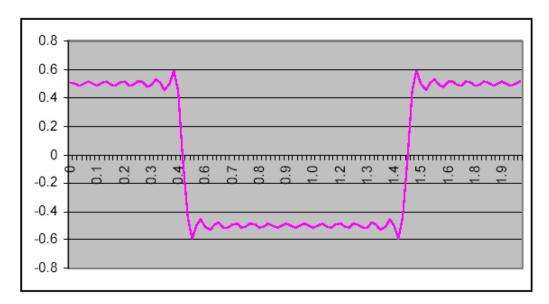
If the lowpass filter has bandwidth 5 Hz, then the first five components are passed (k=4). The resulting signal is shown below:
