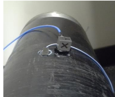
Fig. 3. The tri-axial accelerometer mounted on the receive side.
