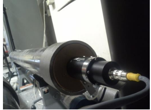
Fig. 2. The transmit transducer mounted along the drill string testbed axis.
