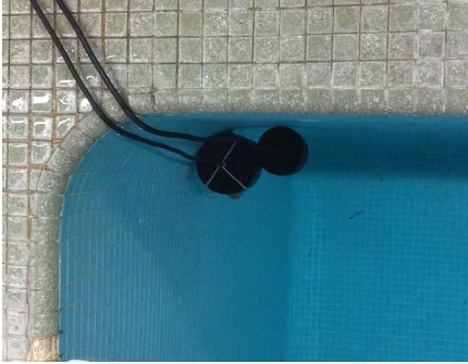
Fig. 1. Vector transmitter of the MISO system includes a ring transducer (left) with four segments which acts as two orthogonal dipoles [1] [2] for two independent data streams, plus a nearly co-located scalar transducer (right) for the third data stream. The transducers are at the same depth and there is no spacing between them.
