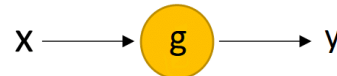
Fig. 1. A single node of neural network. Activation function g(\cdot) maps input x to output y .
