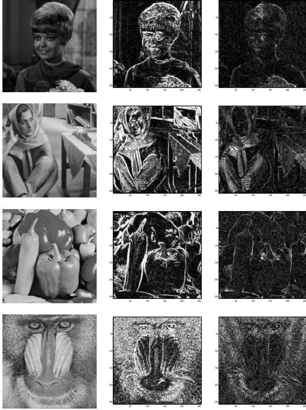
Figure 3: First column : original images. Second Column : Difference between original and StirMarked images. Third Column : Difference between original and unwarped images
