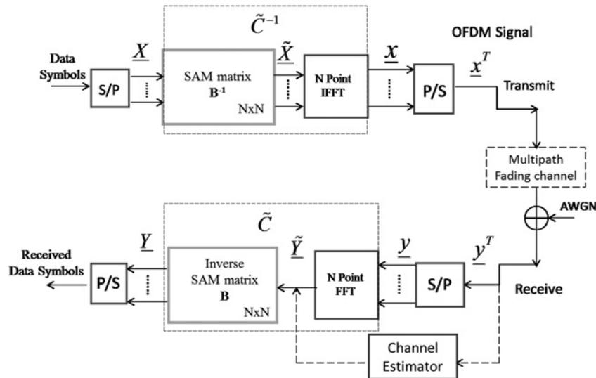
**Fig. 2** Block diagram of the OFDM system with the proposed PAPR reduction method
