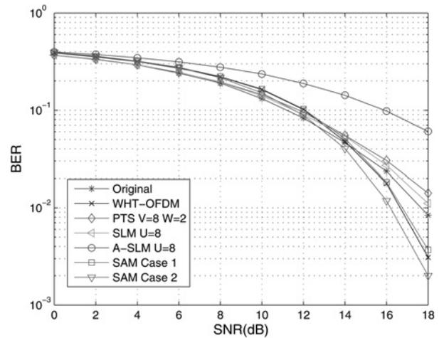
**Fig. 8** BER performance comparisons of the proposed SAM in two cases, WHT-OFDM, PTS, ordinary SLM and A-SLM methods for 16-QAM and  $N = 256$  over multi-path fading channel
