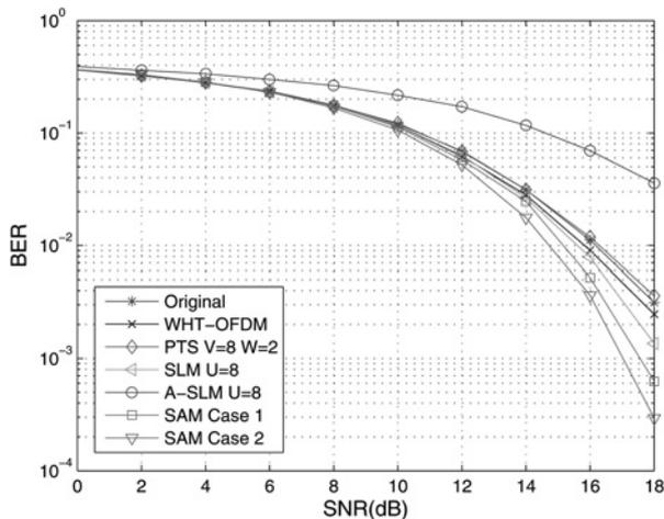
**Fig. 7** BER performance comparisons of the proposed SAM in two cases, WHT-OFDM, PTS, ordinary SLM and A-SLM methods for 16-QAM and  $N = 256$  over AWGN channel
