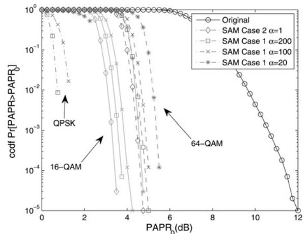
**Fig. 4** PAPR performance of the proposed SAM in two cases for QPSK, 16-QAM, 64-QAM and  $N = 128$  in the OFDM system
