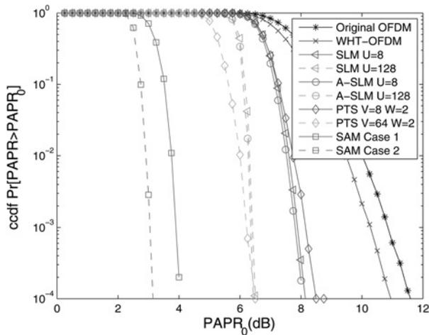
**Fig. 6** PAPR performance of the proposed SAM in two cases, WHT-OFDM, PTS, ordinary SLM and A-SLM methods for 16-QAM and  $N = 256$
