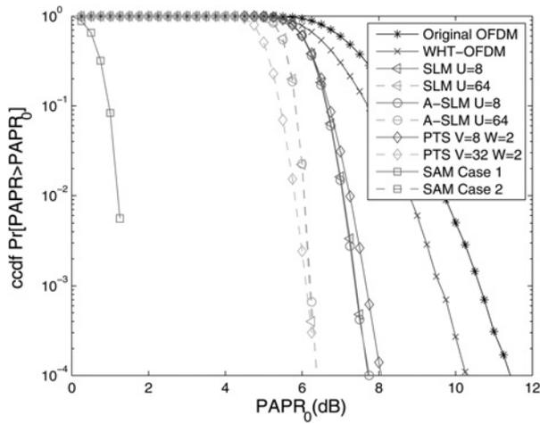
**Fig. 5** PAPR performance of the proposed SAM in two cases, WHT-OFDM, PTS, ordinary SLM and A-SLM methods for QPSK and  $N = 128$
