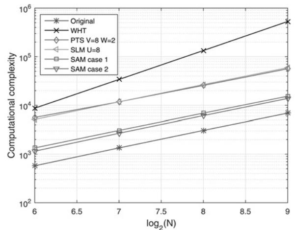
**Fig. 3** Computational complexity of the proposed SAM (two cases), WHT-OFDM, PTS and ordinary SLM methods
