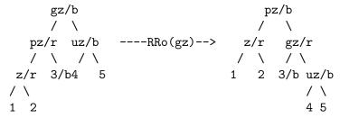
After the single rotation is performed there can be no way that there are two consecutive RED nodes in a path from the root to pz (root of the subtree in Case 3). Therefore after a single rotation we are done.
