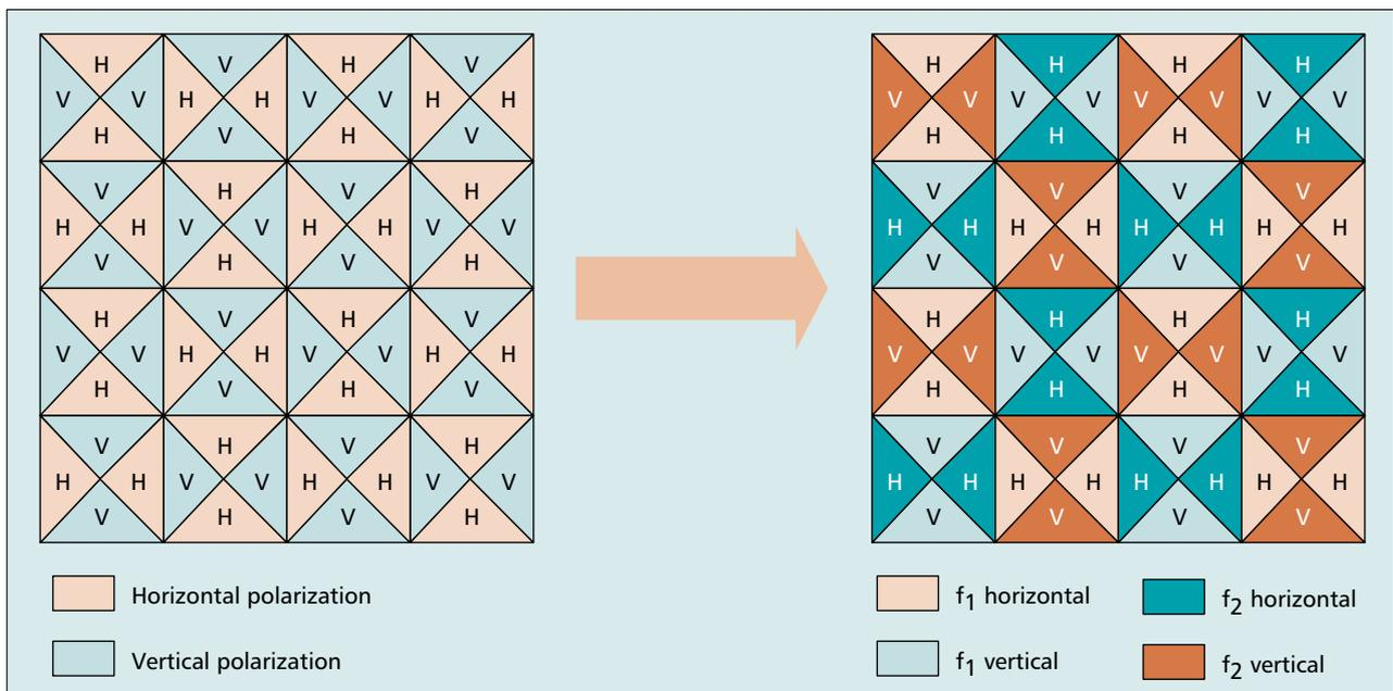
■ **Figure 5.** Alternate polarization between horizontal and vertical, and frequency reuse.
