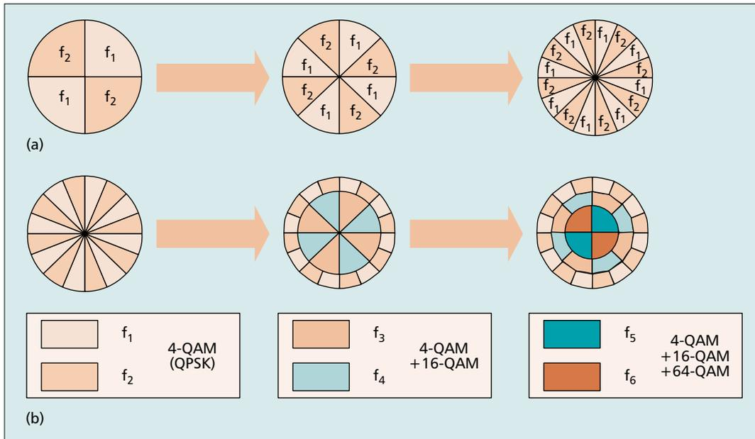
■ **Figure 2.** a) Increasing system capacity by sectorization; b) scalability is achieved by sectorization with multiple modulation schemes. Initial deployment uses 16 QPSK hubs; another eight sectors are increased by adding eight 16-QAM hubs. Further utilization of a full duplex channel can be achieved by adding four more 64-QAM hubs.
