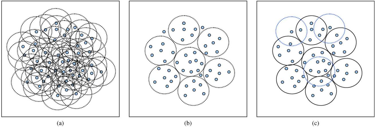
Fig. 4. Proposed clustering procedure. (a) There are  $n$  clusters in the first stage. (b) Chosen clusters by set packing algorithm in the second stage. (c) Clusters added to cover all of the nodes (dotted circles).
