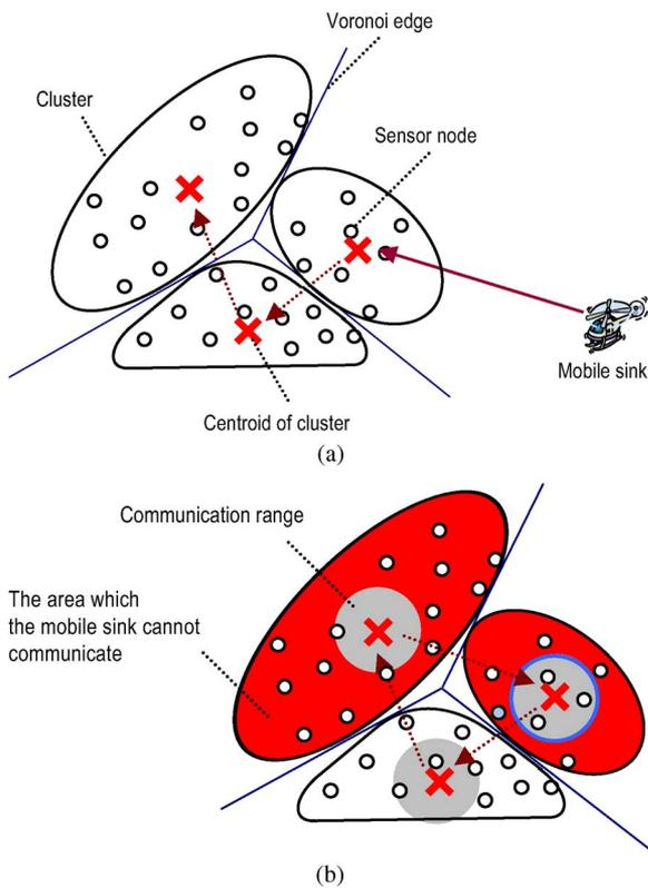
Fig. 3. KAT mobility on WSAN. (a) Overview of KAT mobility. (b) The drawback of KAT mobility.
