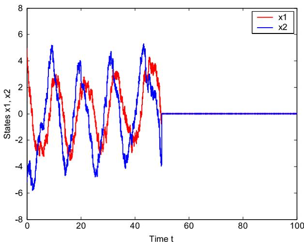
Fig. 8. System response with the control ( $u = \text{Eq. (30)}$  at  $t = 50$ ).
