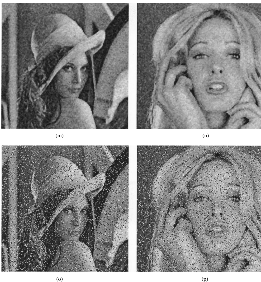
Fig. 3. (Continued.) Experimental results. (m) and (n) are images of (c) and (d) filtered by a 3 \times 3 median filter. (o) and (p) are images of (a) and (b) corrupted by salt-and-pepper noise.
