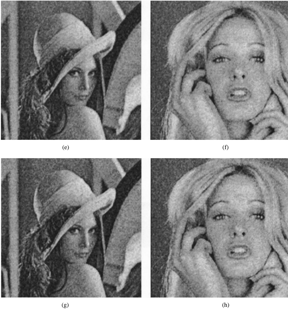
Fig. 3. (Continued.) Experimental results. (e) and (f) are (c) and (d) filtered by a 3 \times 3 linear filter that is configured from (a) and (c). (g) and (h) are images of (c) and (d) filtered by a 3 \times 3 TD filter that is configured from (a) and (c).
