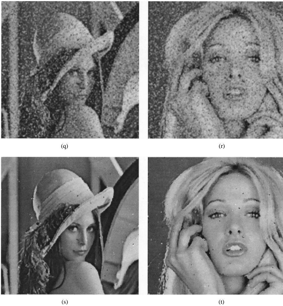
Fig. 3. (Continued.) Experimental results. (q) and (r) are images of (o) and (p) filtered by a 3 \times 3 linear filter that is configured from (a) and (o). (s) and (t) are images of (o) and (p) filtered by a 3 \times 3 TD filter that is configured from (a) and (o).
