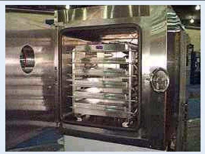
Once secondary drying is complete, shelves are collapsed by a hydraulic ram, to fully stopper the vials.
