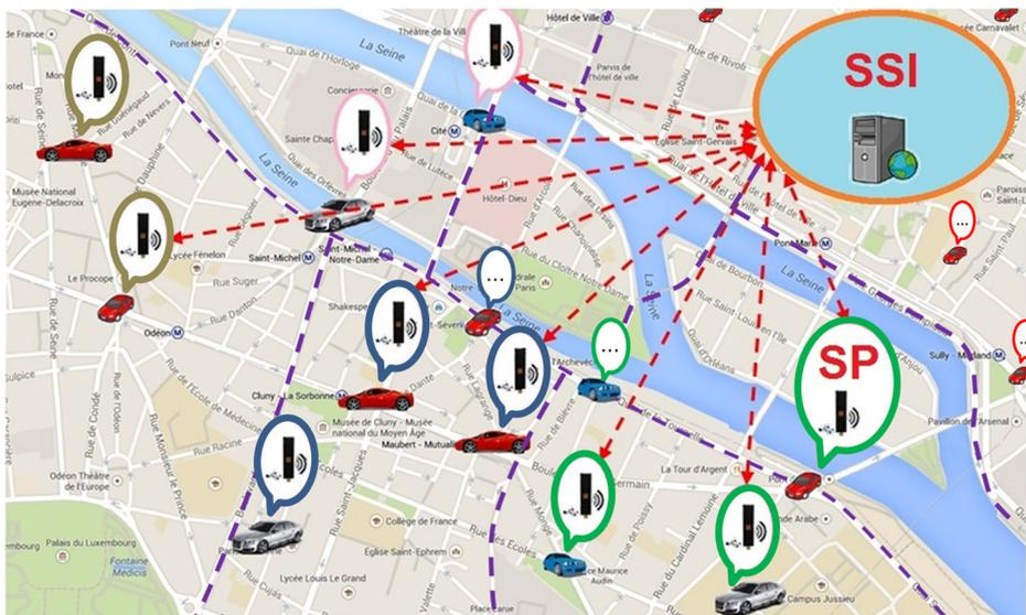
**Fig. 1** Overview of PAMPAS's system architecture: mobile secure probes (SPs) leverage an untrusted Supporting Server Infrastructure (SSI) for efficient message passing among SPs. SPs continuously compute a spatial probe partitioning (depicted by the purple dashed lines) allowing for efficient and secure sample data aggregation
