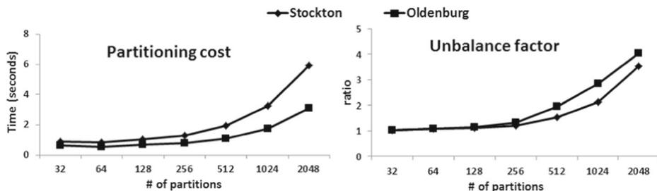
**Fig. 10** The partitioning costs (left) and the partitioning unbalance factor (right) in PAMPAS with different number of partitions
