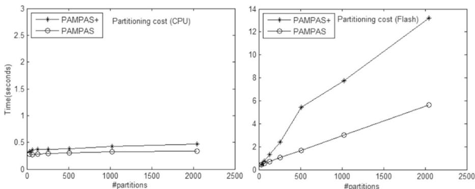
**Fig. 13** The detailed partitioning costs - CPU (left) and Flash IOs (right) - in PAMPAS and PAMPAS<sup>+</sup> with different number of partitions
